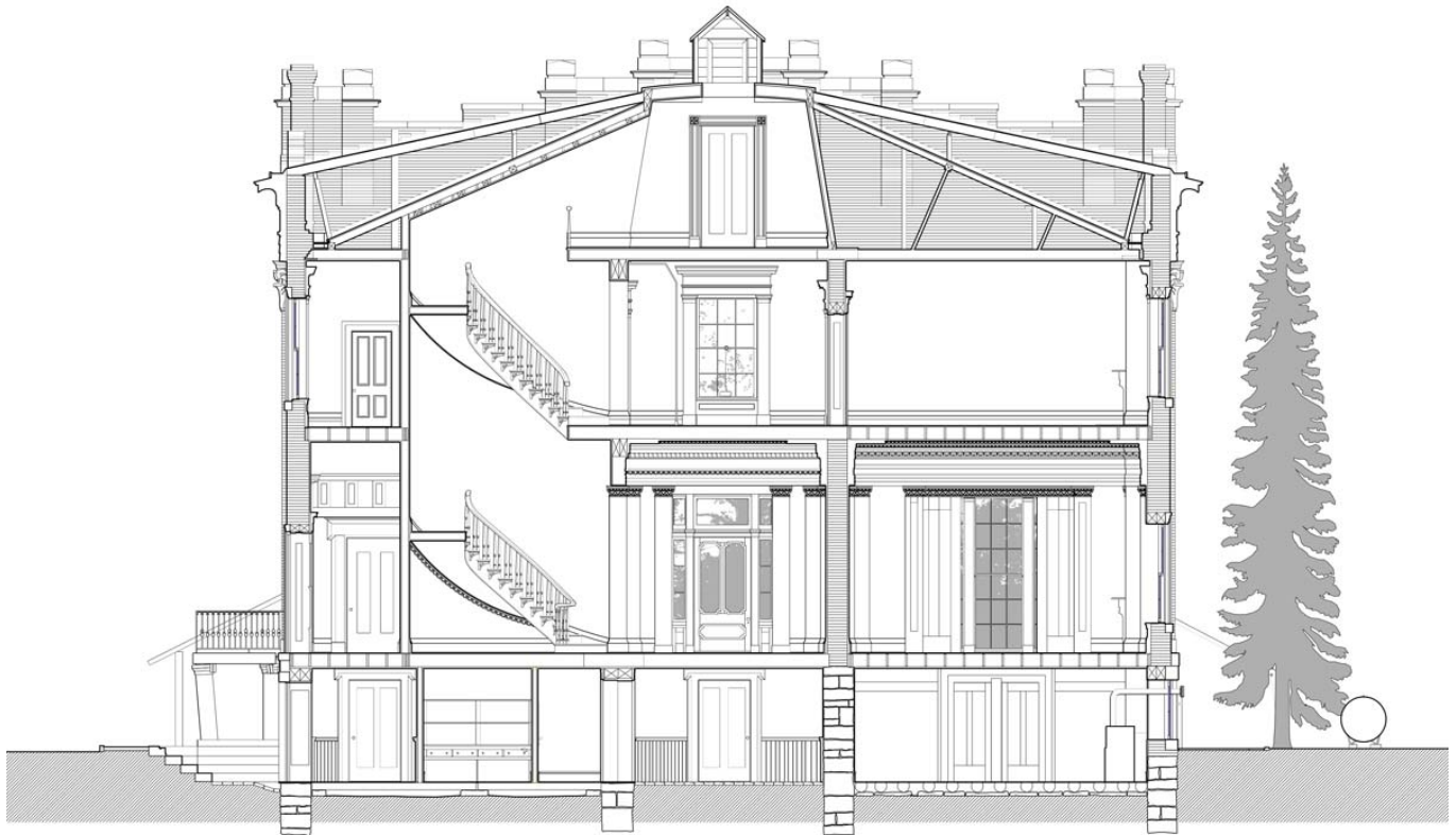
Figure 25. A current condition cross section through the West Entry and the main, nautilus staircase of Ward Hall, looking North . Note the double roofs, the shoring supporting the failed second roof at the chimneys, and the clapboard-sided lantern that has provided little or no light to the Attic landing or, for that matter, the otherwise unlit stairwell, in decades.
